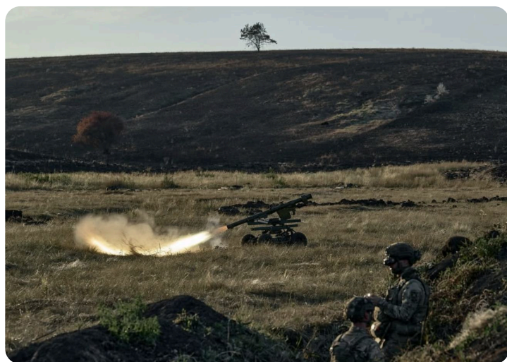
A ground robot with a surface-to-air missile launcher. Source: Kostiantyn Liberov via 28th Mechanized Brigade
