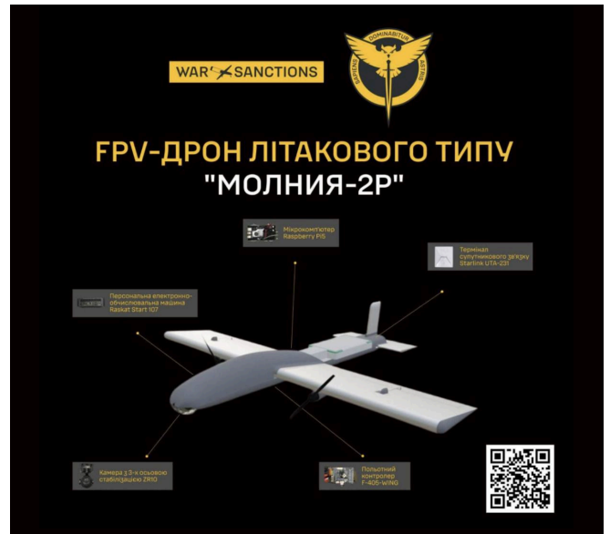
FPV Drone Of The Airplane Type Molniya-2R. Source: Defence Intelligence of Ukraine
