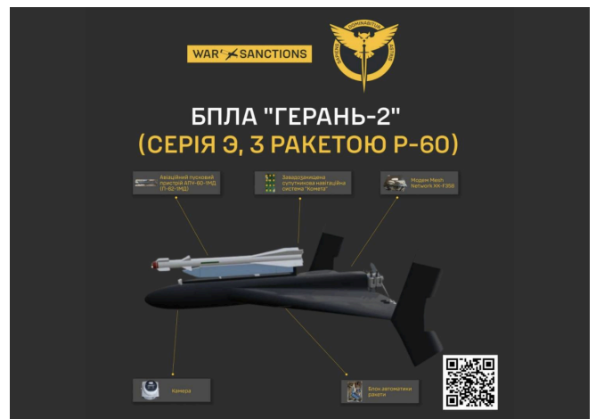
Geran-2 UAV (series "Э", with R-60 missile). Source: Defence Intelligence of Ukraine
