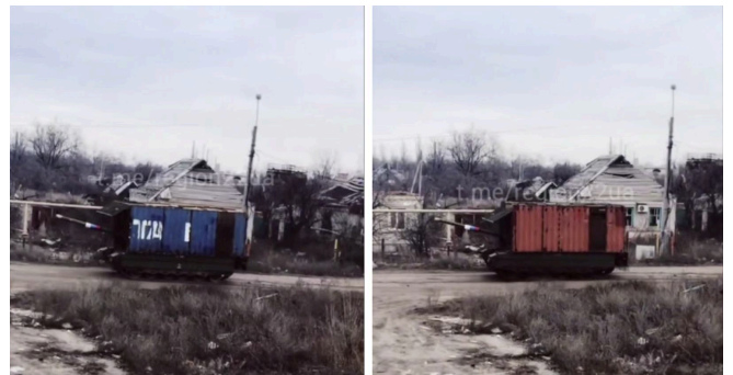
Two Tanks With Maritime ISO Container “Armor”. Source: region22ua
