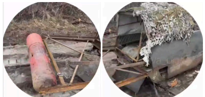
February Protection Configuration of Unknown UGV — “Mangal” and Gas Cylinder Used as Anti-Mine Trawl. Source: texBPLA
