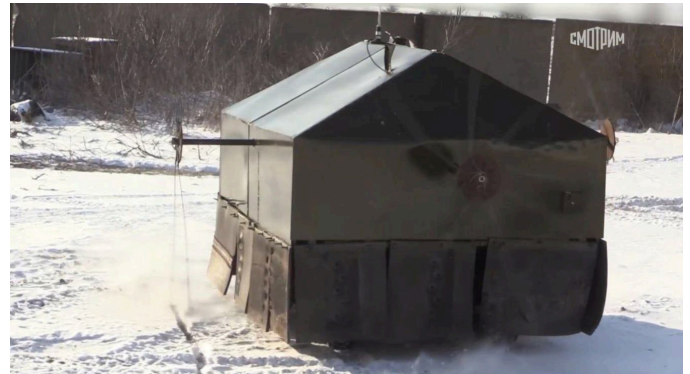
Courier UGV Equipped with Rotating Metal Cables for Anti-Drone Protection. Source: texBPLA
