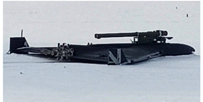
Downed Russian Geran-2 UAV With Integrated Verba MANPADS. Source: serhii_flash
