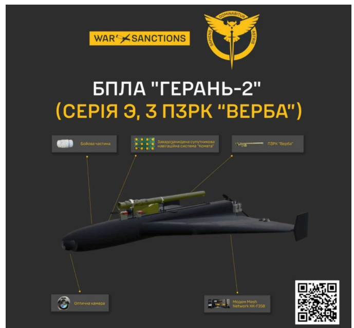
UAV "Geran-2" (Series "E", Equipped With the Verba MANPADS). Source: War & Sanctions
