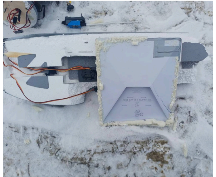
Downed BM-35 UAV With Integrated Starlink. Source: serhii_flash
