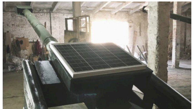
Decoy M777 Howitzer with solar panel. Source: Decoy for frontline «Apate»
