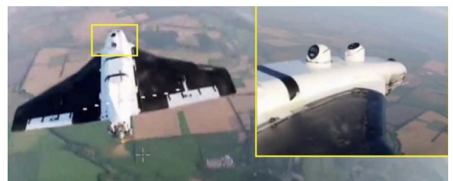
Captured Russian "Gerbera" UAV, equipped with two cameras for visual detection of interceptor drones. Source: Militarnyi
