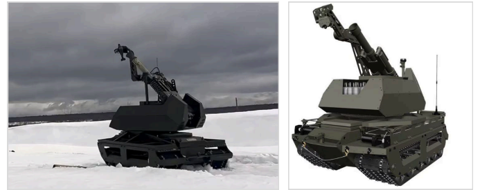
Courier UGV Fitted With an 82mm Mortar and a Robotic Arm. Source: stormdron & texBPLA
