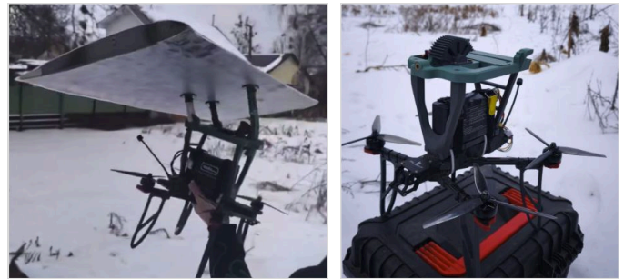
Wing Mount Construction on an FPV Drone. Source: VIUKSIDV
