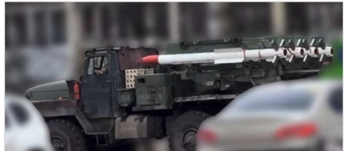
Russian R-77-1 Air-to-Air Missiles Adapted for Ground Launch on Ural-4320 Chassis. Source: mag_vodogray
