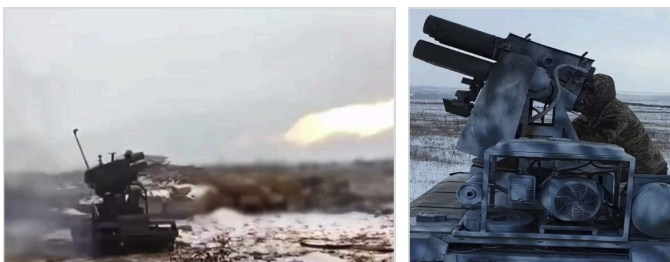
Russian Courier and Impulse UGVs Fitted With Type-75 MLRS. Source: stormdron & Drone Wars
