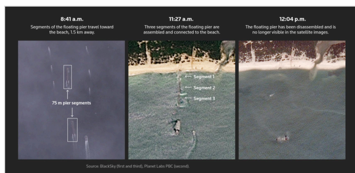
Figure 30. Reuters. A modular floating pier enables temporary shore unloading without a functioning port. 94
