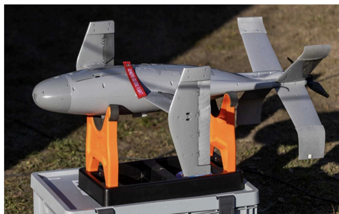
Figure 61. Militaryni . Surveyor interceptor drone of the Merops anti-drone platform 134 .
