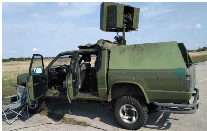
Figure 57. Militarnyi . Bukovel-AD electronic warfare system mounted on an off-road vehicle chassis. 2019 126 .
