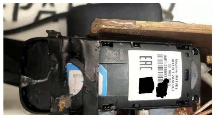
Figure 29. Modem and a SIM card of the Ukrainian mobile operator Kyivstar installed on the body of a Shahed UAV.
