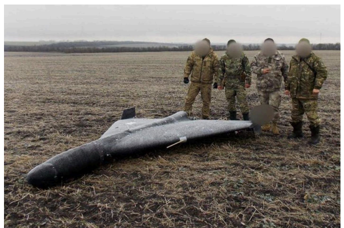
Figure 58. Militarnyi . Neutralized Shahed UAV over Ukraine as a result of electronic warfare activity 129 .
