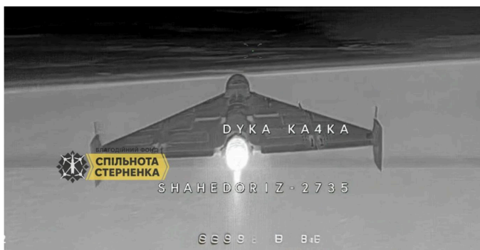
Figure 36. Serhii Sternenko Foundation. Shahed-238 jet-powered UAV (Geran-3) 68 .
